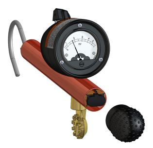
Check meter, battery and circuitry for proper operation before and after each use by depressing test button at back of meter housing while switching selection to each setting in sequence. Set at every position except "Off", meter should read nearly full scale. When reading falls three or four divisions below full scale, replace battery by removing plastic cap on end of mounting stick. Use a 9-volt battery.
